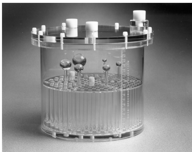
Components of Deluxe Jaszczak Phantom™
